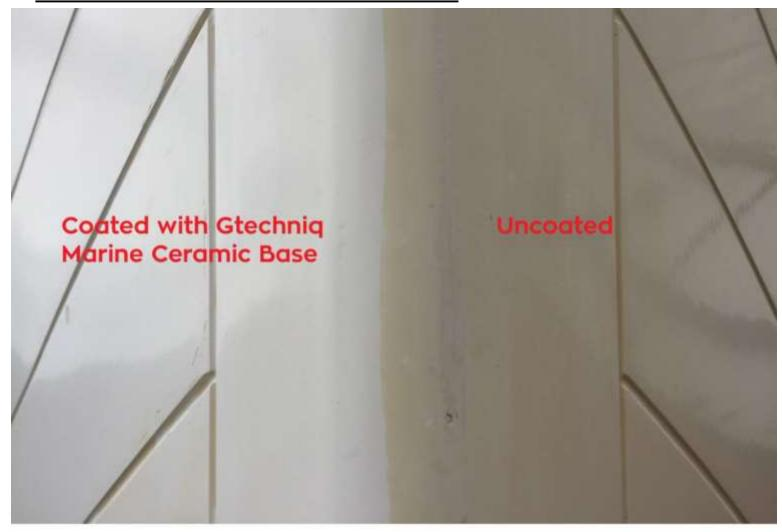
This picture is of the bow of a fiberglass trawler. GT Marine Ceramic Base was applied to the left side and the right side had no coating applied. The trawler operates in Desolation Sound, British Columbia, a waterway that has a very high level of tree sap that easily stains gelcoat. This photograph was taken 1 year after application.
